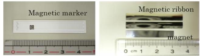
Fig. 5 Photograph of the resonated marker.
