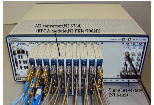
Fig. 4 Photograph of the PCI eXtensions for Instrumentation (PXI) system. 40 AD converters (NI 5734), FPGA modules (NI PXIe-7962R) and signal generator (PXI-5402) were set in the chassis.
